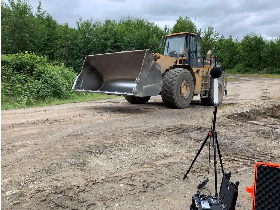
Figure A1. Typical Noise Measurement Setup
